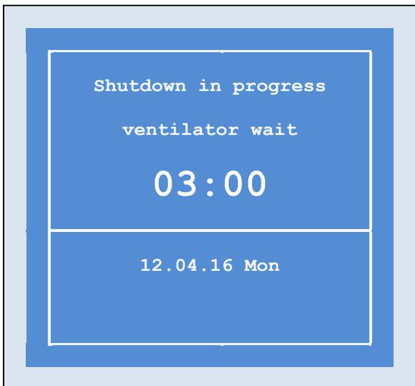
When pressing oven off switch, the display shows the post-ventilation time counting, after which oven switches completely off.
