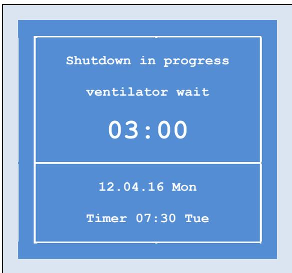
The 3-minutes time of post-ventilation is set by "408" parameter. To change it just edit value of this parameter, see chap. "Settings-Users parameters"
